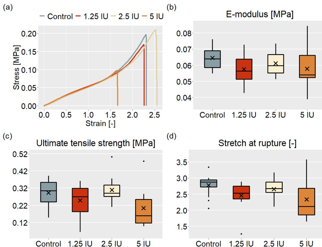
**Figure 3.3. The mechanical characteristics of L-PRF membranes.** (a) A representative stress-strain curve, (b) the E-modulus, (c) the ultimate tensile strength, and (d) the stretch at rupture are shown. The mean (X) is indicated. The control (without enoxaparin), 1.25 IU, 2.5 IU, and 5 IU enoxaparin-supplemented L-PRF membranes were compared.
